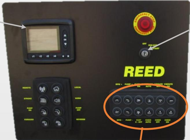
**RPM +/-** controls increase and decrease of engine RPM. It will be backlit when each function is engaged.
