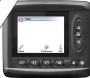
4. Main Menu Screen - After pressing the menu button a screen appears that provides the operator three options Adjust, Preferences, and Info
