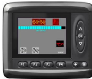
3. Scrolling Screens – Providing a Straight forward convenience for the operator and easier access to pump status items using the up and down arrows to scroll through the primary operational and status displays.
