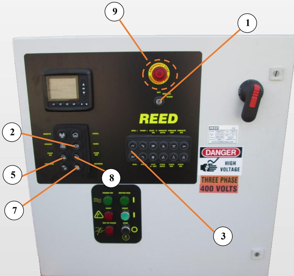
1. Turn KEY operated SYSTEM POWER Switch to “ON”
