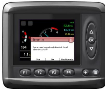
2. **PROX OVERRIDE MODE** - Select **Override** from the popup (above) **Stroke** button will be flashing to indication **Override** mode. (Below)
