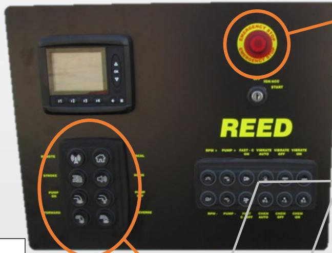
**CONTROL SWITCH (LOCAL/REMOTE)** this is used to select the pump control location. Press button to **LOCAL** to enable operation of concrete pump for main stationary panel. Press button to **REMOTE** for operation using the remote control. It will be backlit when each function is engaged
