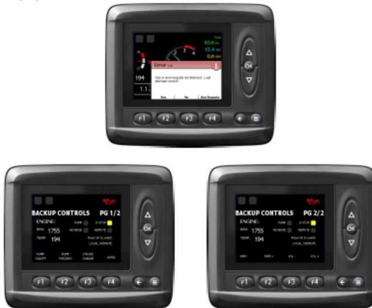
3. ALTERNATE CONTROL MODE - Selecting REMOTE when there is an error will allow normal remote controls. Pressing the OK Button toggles REMOTE and LOCAL.
