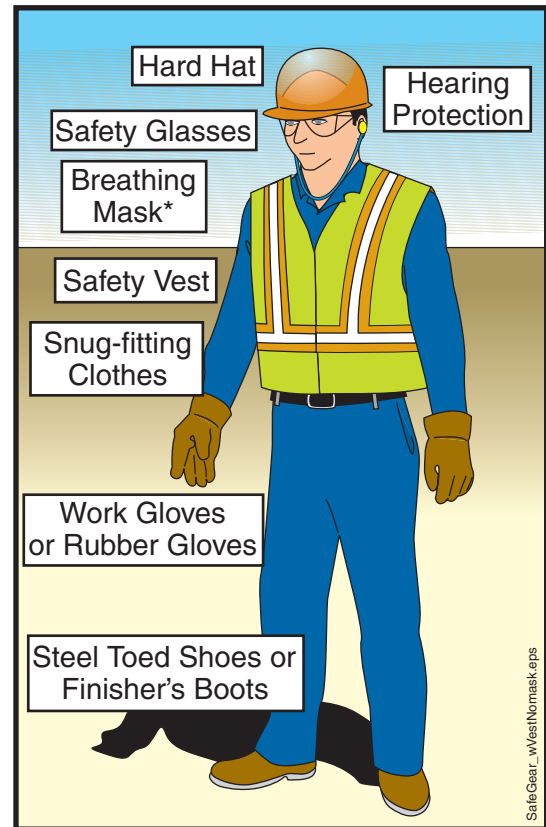
Figure 1 Personal Protective Equipment (P.P.E.)
