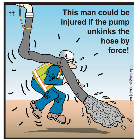
Figure 49 Kinking the hose creates a hazard
