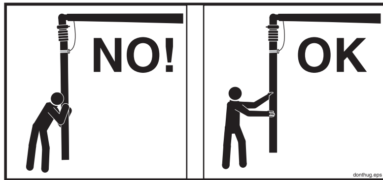
Figure 84 Do not hug the boom hose
