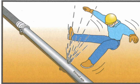
Figure 9 Delivery system components must be able to withstand maximum pump pressure
