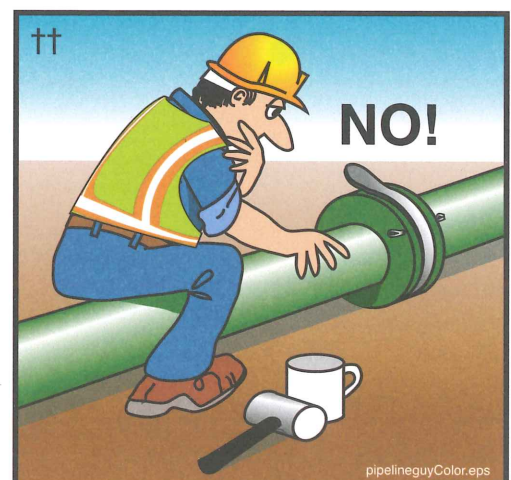
Figure 54 Never straddle or sit on a pressurized pipeline
