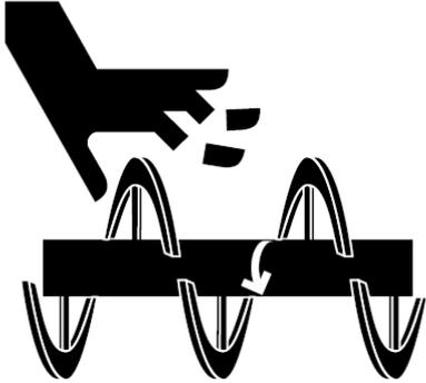
Keep hands out of hopper and valve assembly. See operation manual if access is required.
