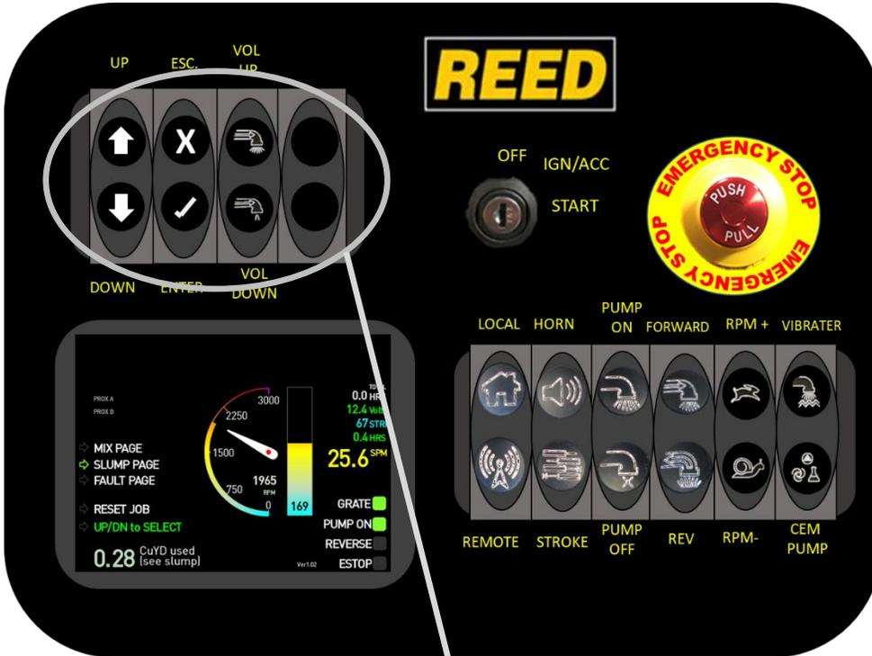
1. PUMP VOLUME, this is to turn the pump volume up or down. Press button **VOLUME UP** to increase volume, and press button **VOLUME DOWN** to reduce volume.
