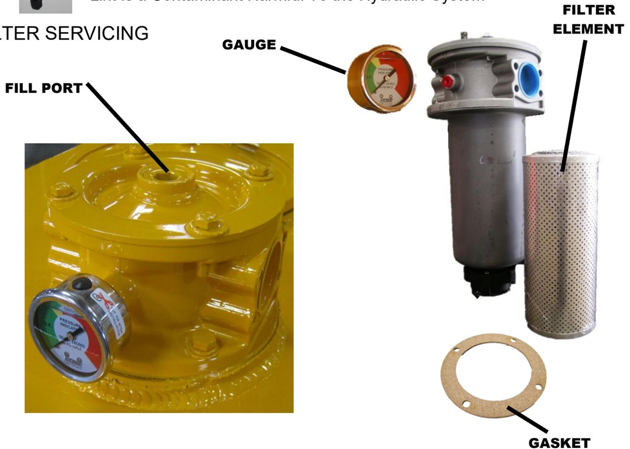
Hydraulic filters provide a means of continuous hydraulic fluid filtration in an effort to prevent recirculation of contamination which will cause rapid wear and component
