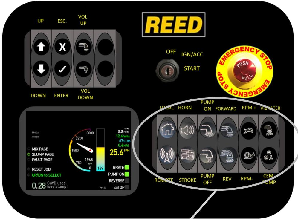
1. **CONTROL SWITCH (LOCAL/REMOTE)** this is used to select the pump control location. Press button to **LOCAL** to enable operation of concrete pump for main stationary panel. Press button to **REMOTE** for operation using the remote control.
