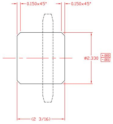
1.MADE FROM C-9K108 SPROCKET, REMOVED FROM FRONT OUTRIGGER.
