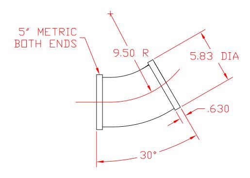
CONFORMS #188M11012H OLD PART NUMBER, NO LONGER MANUFACTURED CONFORMS #265M11012 NEW PART NUMBER
