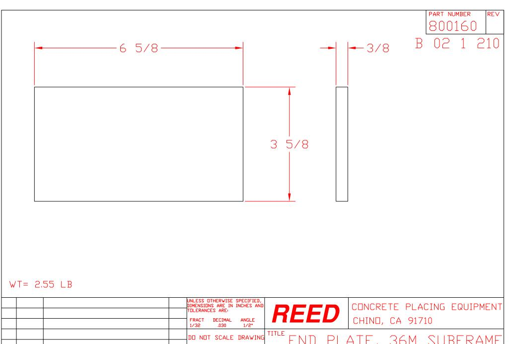
END PLATE, 36M SUBFRAME CE PART NUMBER REV MATERIAL #68190 FLAT 3/8 X 4 HRS BY DATE 800160 THIS DRAWING IS THE PROPERTY OF REED MANUFACTURING AND IS DRAWN JIM0 7/28/97 LOANED WITHOUT CONSIDERATION OTHER THAN THE BORROWER'S LTR DATE ENGINEERING CHANGE NOTICE # BY AGREEMENT THAT IT SHALL NOT BE REPRODUCED, COPIED, LOANED OR DISPOSED OF, DIRECTLY OR INDIRECTLY, NOR USED FOR ANY REVISIONS SHEET\_\_OF\_\_ APPVD PURPOSE OTHER THAN THAT FOR WHICH IT IS SPECIFICALLY
