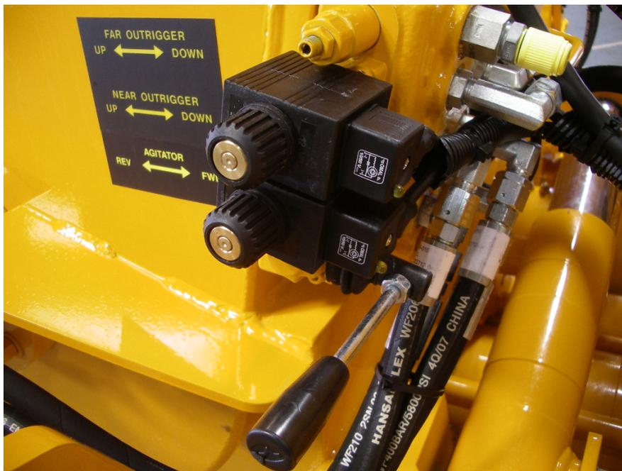
AGITATOR CONTROL controls agitator ON/OFF and FORWARD REVERSE functions.
