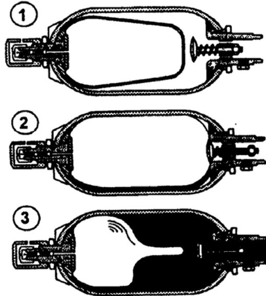
**MORE DETAILS:****1. Empty accumulator Without precharge****2. Accumulator precharged, no oil charge**
