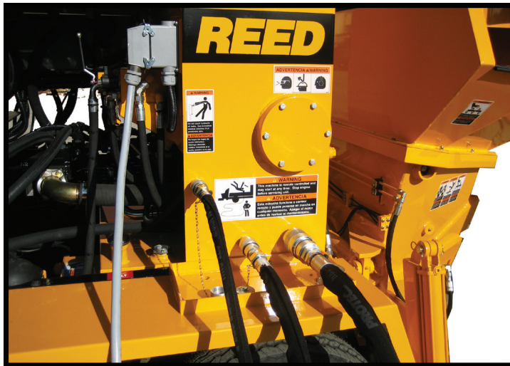
REED M2200 Pan Mixer being powered by the REED P50 Electric/Hydraulic Power Pack (P50 slides under M2200 for easy transport)
