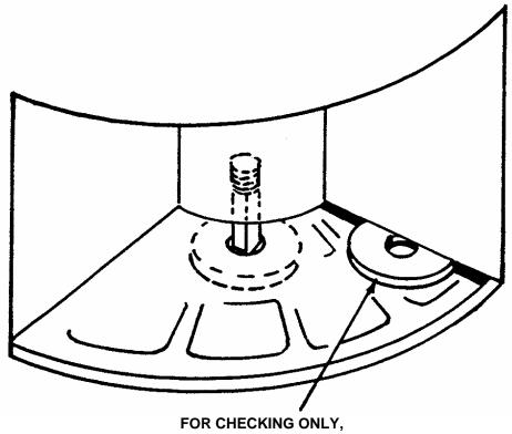
FOR CHECKING ONLY, IF THIN RISER PLATE SLIDES IN HERE, RISER PLATE SHOULD BE PLACED UNDER FEED BOWL.
