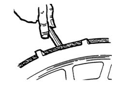
FELT SEAL BEING ADJUSTED TO WEAR PLATE
