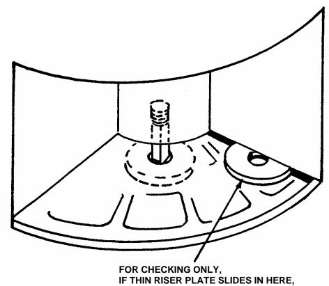
RISER PLATE SHOULD BE PLACED UNDER FEED BOWL.
