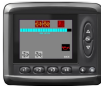
DEF TANK LEVEL
