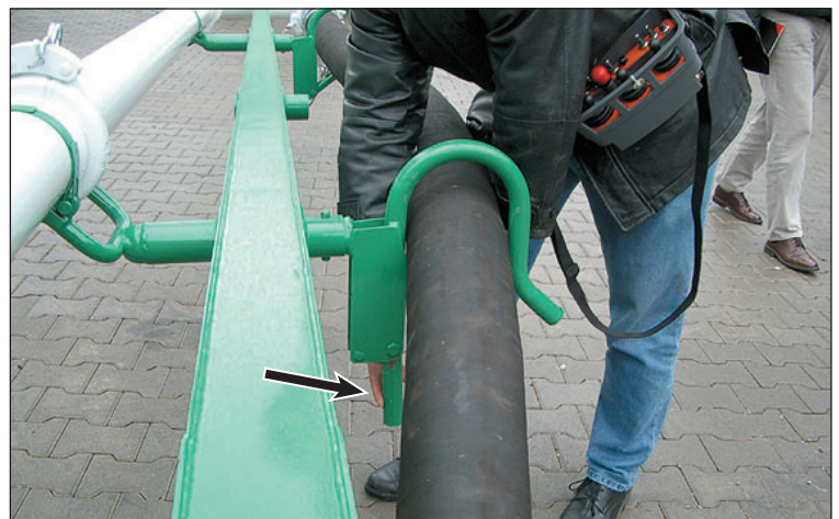
Fig. 7.17 Release the discharge hose
