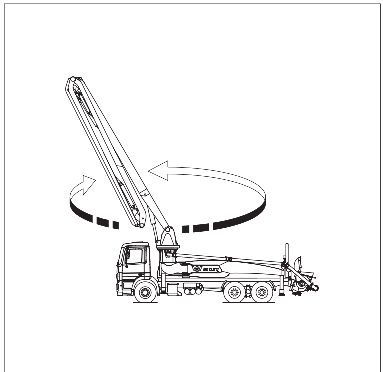
Fig. 7.13 Slew the boom package into the working position
