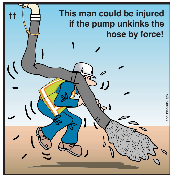
Figure 86 Never kink the hose; Never hold the hose with your shoulder
