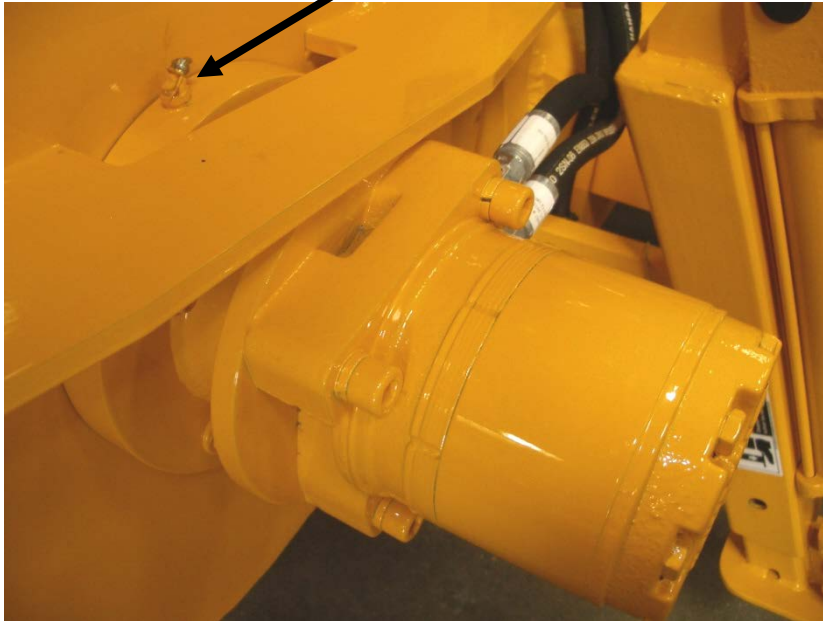
HYDRAULIC MOTOR SIDE GREASE POINT
