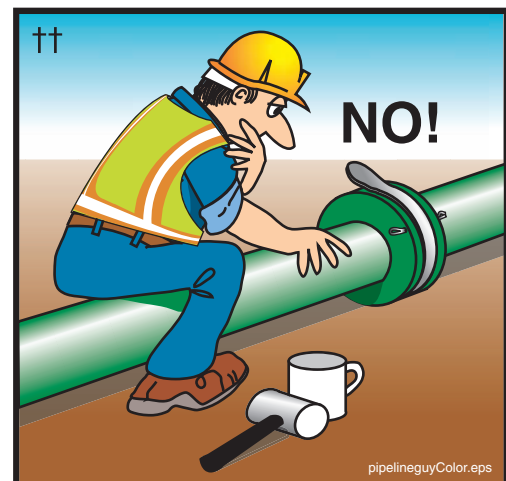
Figure 88 Never straddle or sit on a pressurized pipeline
